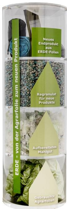
*Fig. 3. From agricultural film waste to new film – the ERDE Recycling initiative paves the way by ensuring that used agricultural films are recovered and recycled in an environmentally-friendly way.*
